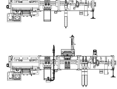
Line expansion brings greater flexibility and efficiency: Machine layout for vial application and after expansion (vial and/or syringe application) and an additonal bookletfeeder
