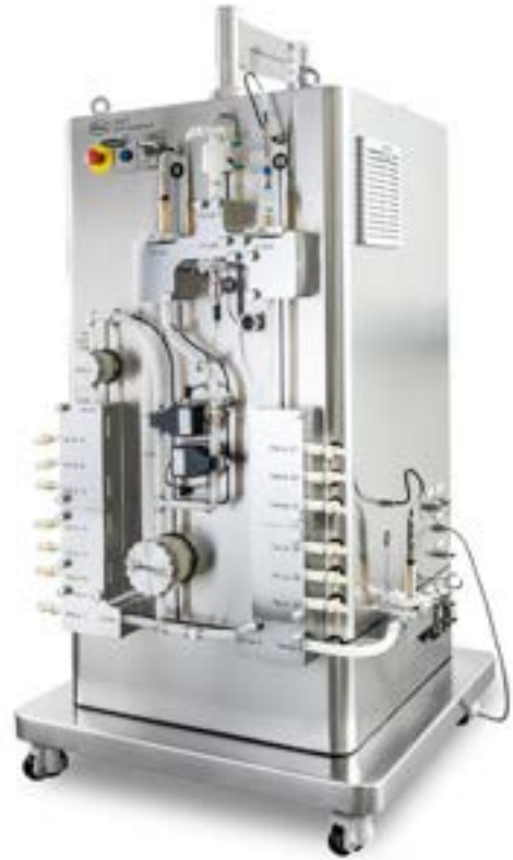
Installed single-use manifold
